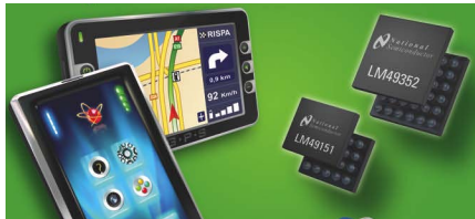
The low-power LM49352 audio codec for handheld consumer electronics has Class D-amplifier outputs.
