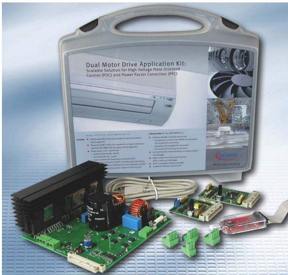
The dual-motor-drive-application kit supports FOC and power-factor control with a scalable architecture from 8 to 16 bits and a power board driving as much as 8A at 110 to 230V.
